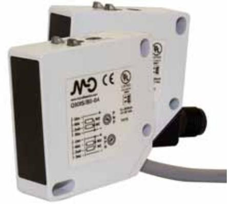
The new series of **Photoelectric Sensors Q50**, size of **50 x 50 mm**, includes a wide range of versions: **Direct Diffuse model with working distance up to 2 m**, **Background Suppression model up to 500 mm**, **Polarized Retro Reflective model up to 6 m** and a **through-beam version (emitter and receiver) with sensing range of 20 m**.
